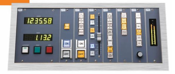
Turret Panels can be used for a wide variety of functions, and are typically installed at host, co-host and guest positions. 6" high x 1.6" wide. Mounting rails are available in any width for integration into your studio furniture. SAS Turret Panels interface to the 32KD or RIO via RS485 serial, four modules to a single RS485 port. 12VDC.
