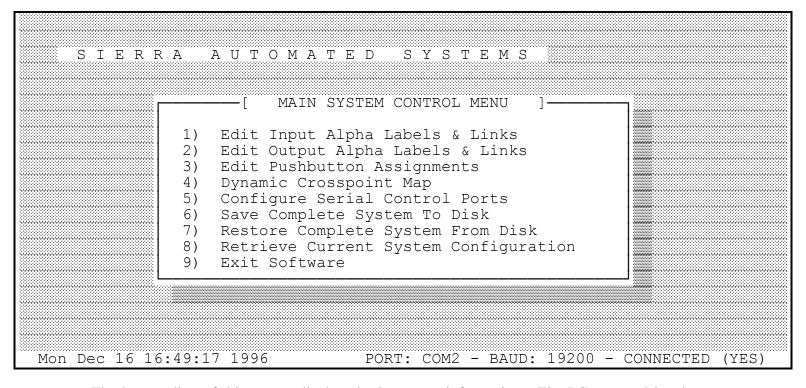
The bottom line of this screen displays basic system information. The PC port and baud rate (always 19200 baud) are shown and the communication status of the PC to MCU link is displayed. If the serial communication is disrupted the (YES) will immediately reflect (NO).
