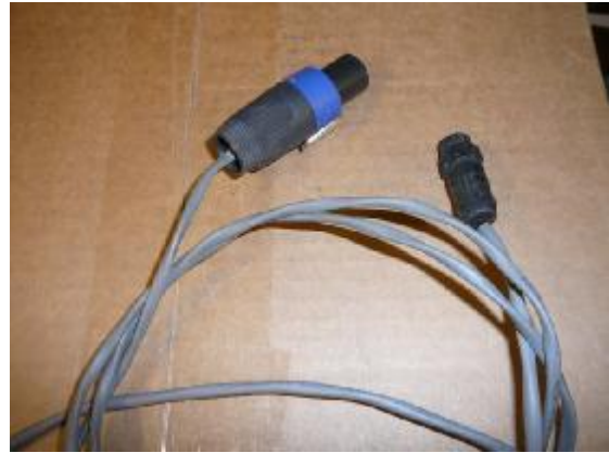
Meter Bridge Power Cable
