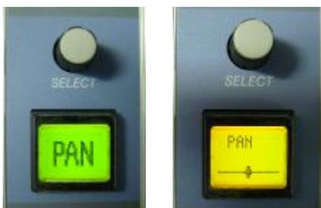
Pressing the knob after dialing up the PAN menu brings up the display on the right. Turning the knob now will pan the audio left or right.
