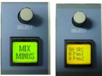
The mix-minus menu is two pages deep. The first press of the select knob after scrolling to MIX MINUS brings up the ON Source screen. The upper source name (A Pgm1 in this example) is the currently selected mix-minus base-bus when the input module is turned ON. If you want to change this base-us, dial up a different bus or source (the lower source name will scroll through) and press the MFD to select.
