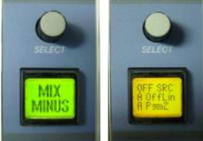
When you're done with the On Source, press the Select knob again and you'll get the OFF Source screen. The upper source name (A OffLin in this example) is the currently selected mix-minus base-bus when the input module is turned OFF. If you want to change this base-us, dial up a different bus or source (the lower source name will scroll through) and press the MFD to select.
