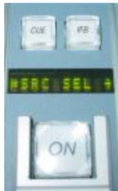
The display shows the available sources (as determined by engineering) as you turn the knob. Pressing the TAKE button (flashing to indicate that the source is pending) will select the new source for the fader to control. The old source is simultaneously removed from whatever busses it was assigned to. Engineering may opt to disable source selection when a current source is turned on, or altogether, on a fader by fader basis.
