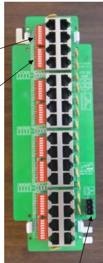
Power input connector for 12VDC.
