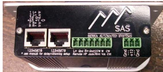
Fig 2. The back-panel connections
