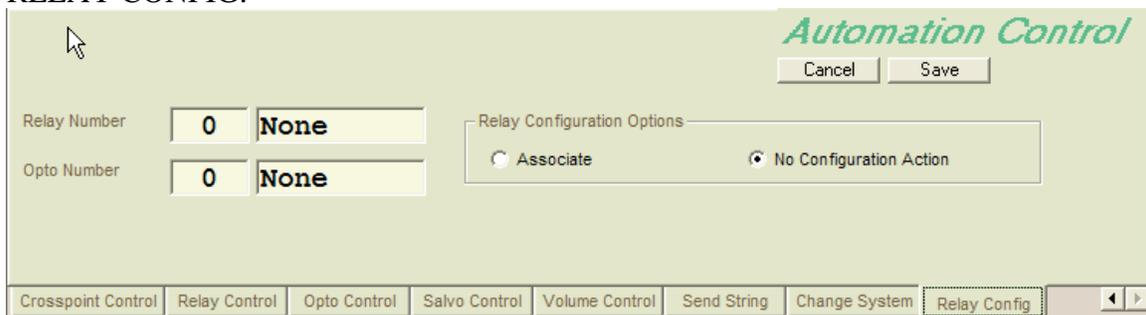
The screenshot shows the 'Automation Control' software interface with the 'RELAY CONFIG' dialog box open. The 'Relay Number' is set to '0' and 'None'. The 'Opto Number' is set to '0' and 'None'. The 'Relay Configuration Options' section has 'No Configuration Action' selected. The bottom navigation bar includes buttons for 'Crosspoint Control', 'Relay Control', 'Opto Control', 'Salvo Control', 'Volume Control', 'Send String', 'Change System', and 'Relay Config'.
