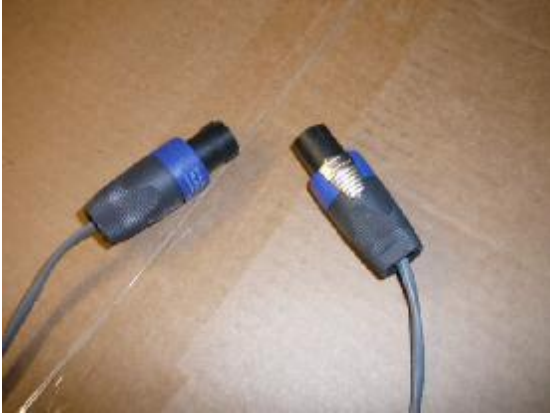
Standard DC Power Cable for RIO (SPR200 Cable shown)
