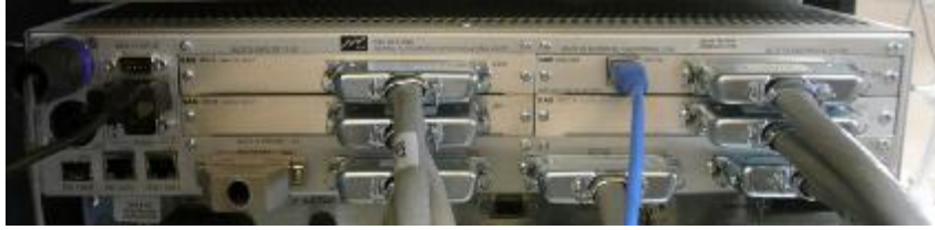
Figure 2. RIO rear panel connections.
