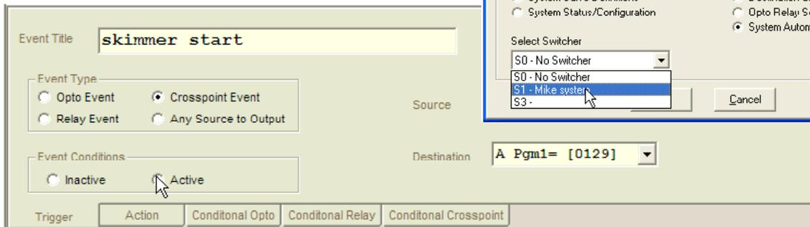
**Any Source to Output:** Here you specify a destination and the event conditions. If the Event Condition is ACTIVE, the trigger occurs if any source is routed to the specified destination. If the Event Condition is INACTIVE, the trigger occurs when the output is cleared (has no source routed to it).
