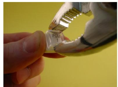
Sometimes a greenie helps, but usually you can grasp the base, and pull the lens off gently with the pliers.
