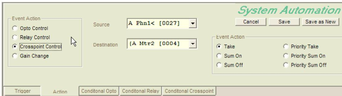
Selecting Crosspoint Control in the Event Action Box allows you to perform crosspoint controls when the event's trigger conditions are met.
