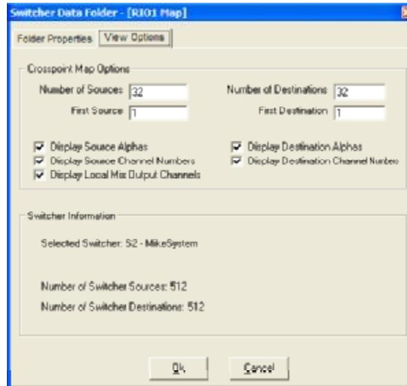
Figure 5. Adding Local mix Output channels (DSP loopback sources) to the map.
