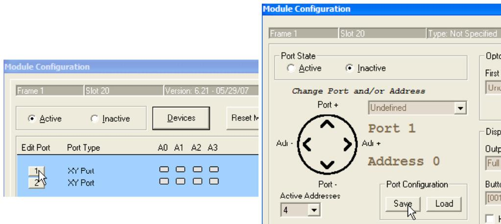
Click on one of the numbered ports. Then click on the Save Port Configuration button. The filename will be Module0120.cfg if the module is in slot 20 of frame 1. Leave this filename as it is and click Save. The file contains settings for the rs485 ports on the card.
