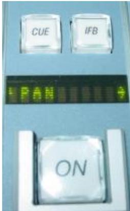
Pressing the knob after dialing up the PAN menu brings up the display on the right. Turning the knob now will pan the audio left or right. Be aware that PAN is a real-time control, taking effect as you turn the knob. Pressing TAKE while panning will immediately jump the pan setting back to center.
