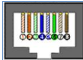
Figure 5: RJ45 Wiring Diagram TIA/EIA 568B Standard
