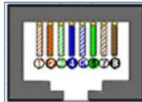
Figure 5: RJ45 Wiring Diagram TIA/EIA 568B Standard
