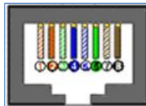
Figure 5: RJ45 Wiring Diagram TIA/EIA 568B Standard
