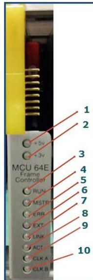
Figure 1: MCU-64 Front Panel
